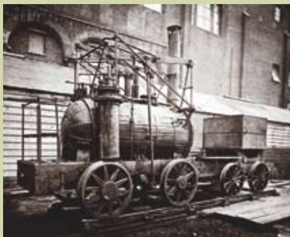
William Hedley developed the system that gave locomotives with smooth wheels sufficient traction. He patented this in 1813, the same year he unveiled his famous steam locomotive, "Puffing Billy," here seen outside of London's Patent Museum (today's Science Museum).
