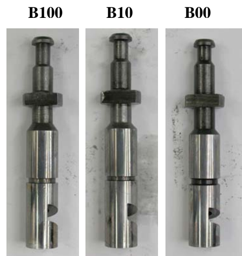
Fig.6: The change in weight and photographs of plunger after the test.
