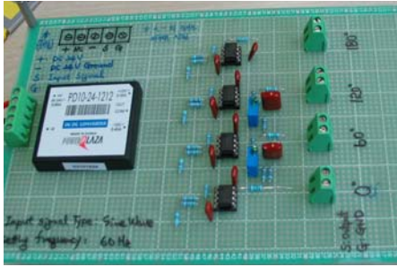
Fig. 3. Multi-phase shifter with the range of 0^\circ to 180^\circ .
