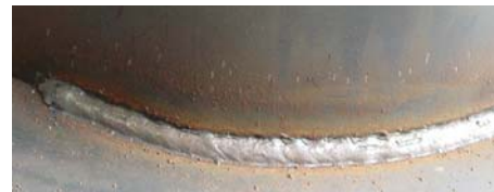
Photo. 5 Welding results of DDWM
