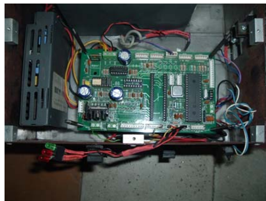
Photo 2. Control board of experimental robot In this diagram, the main control board uses two chips PIC18F458, one gets information from
