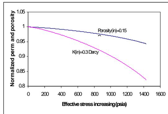
Fig. 3: Normalized permeability and porosity (current by initial) plotted as function of effective stress. The initial porosity and permeability values are given.
