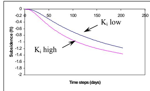
Fig. 2: Subsidence due to production at center sink.  $K_i$  = initial permeability.
