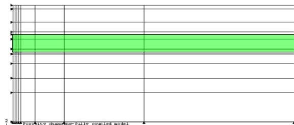
Fig.1: The axisymmetric well model used. Green highlight indicates the production zone.
