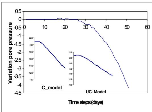
Fig. 4: Difference between the pore pressures for uncoupled minus the coupled models plotted against production time ( $\Delta P = \Delta P_{uc} - \Delta P_c$ )
