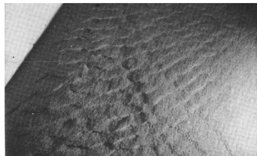
Photo.4 Linguoid ripples I=1/284, Q=8.4l/s, h_m =2.21cm
