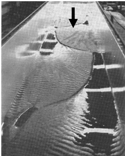
Photo.5 Alternating barsI+ RipplesII I=1/133, Q=6.11/s, hm=1.78cm
