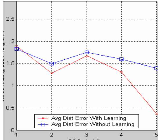
Figure 6: The distant errors of the mobile target versus the number of recursions
